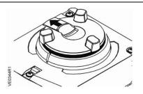
When the black slide switch is pushed out, the manual adjuster remains engaged.
