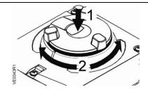
When pushing the manual adjuster down (1), it engages and the actuator can be manually operated.
