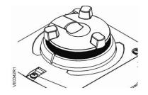
When the motor drives the manual adjuster turns. In Automatic Mode, the manual adjuster is used for indication of travel. If the manual adjuster is held firm in this mode, there is no transmission of power to the gear train.
