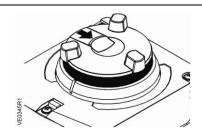
When the black slide switch is pushed back in, and the manual adjuster is not pressed down, the manual adjuster returns to Automatic Mode.
