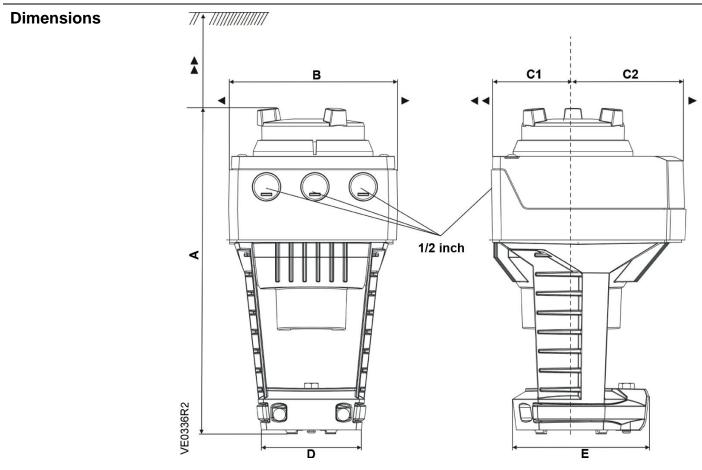
Figure 5. Dimensions in Inches (Millimeters).
