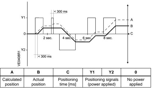
Figure 1. Three-position (Floating) Actuator Deviation.
